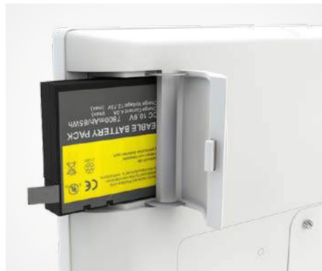
Easily hot-swap battery packs in a matter of seconds
